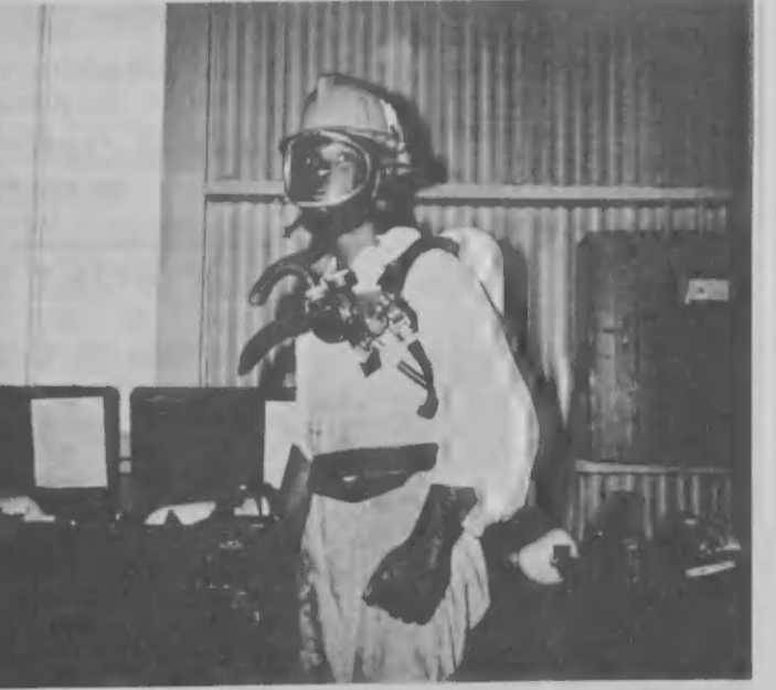
THIS SCOTT-AIR-PAK gas mask is used for protection against high concentration of gas, smoke and dust.
